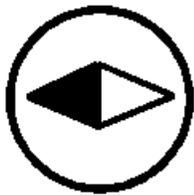
This symbol indicates the map with the vehicle travel direction up, known as Heading Up mode. The shaded triangle indicates the North direction. While in Heading Up mode, the direction your vehicle is traveling will always be at the top of the map screen. The vehicle icon will always be headed in the direction your vehicle is traveling. Touch this screen symbol to switch between Heading Up and North Up modes.
