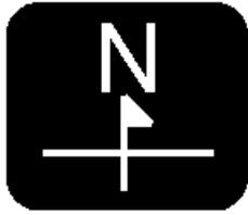
This symbol indicates the map with North Up, known as North Up mode. While in North Up mode, North will always be at the top of the screen. Touch this screen symbol to switch between North Up and Heading Up modes.
