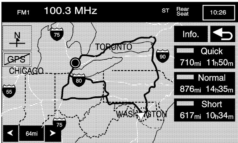
The system will calculate up to three different versions of your current route in three different colors: Quick, Normal, and Short. The routes are shown with distance to destination and estimated travel time. Touch the button corresponding to the route you want to choose.
