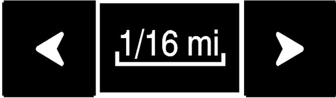
To view a larger or smaller scale of the map, touch the map scale arrows. You can change the level of map detail by either zooming in or zooming out using the arrow screen buttons or by touching the scale on the bar. The system will adjust the map accordingly. The scale of a map can range from 1/32 of a mile (0.05 km) to 128 miles (256 km).
