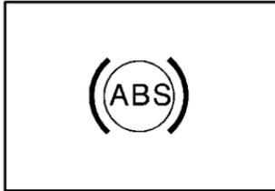
With the anti-lock brake system, the light will come on when you start your engine and may stay on for several seconds. That's normal.
