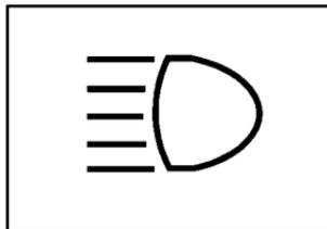
When the high beams are on, this light on the instrument panel cluster also will be on. To change the headlamps from high to low, pull the lever rearward.
