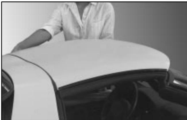
8. Stand on one side of the vehicle and, if necessary, have your helper stand on the other side. Together, carefully lift the front edge of the panel up and forward, and out of the vehicle opening.
