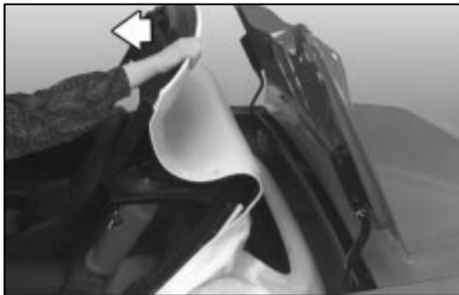
2. Tilt the driver's seat forward and press the storage compartment release button, or use the manual release cable if battery power has been lost. Lift the storage compartment lid (C). (After pressing the release button, the driver and passenger door glass should retract to the full-down position, if they have not already been lowered.)
