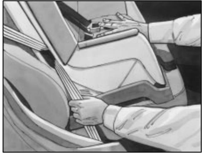
6. To tighten the belt, feed the lap belt back into the retractor while you push down on the child restraint. You may find it helpful to use your knee to push down on the child restraint as you tighten the belt.
