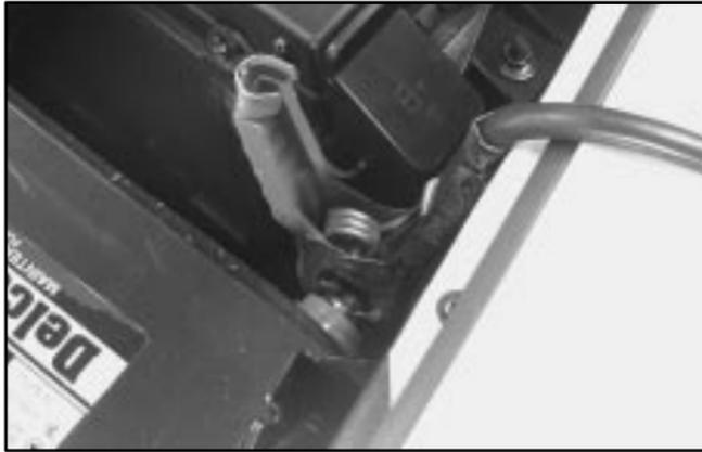
6. Positive (+) goes to positive (+) and negative (-) goes to a heavy, unpainted metal engine part. Connect the red positive (+) cable to the positive (+) terminal of the vehicle with the dead battery. Use a remote positive (+) terminal if the vehicle has one.
