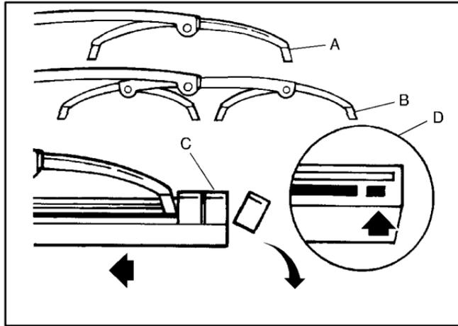
1. Slide the insert (D), notched end last, into the end with two blade claws (A). Slide the insert all the way through the blade claws at the opposite end (B). Plastic caps (C) will be forced off as the insert is fully installed.
