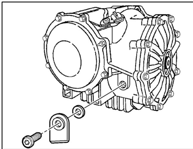
If the level is below the bottom of the filler plug hole, you'll need to add some lubricant. Add enough lubricant to raise the level to the bottom of the filler plug hole.
