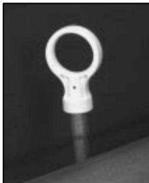
The engine oil dipstick is located near the coolant surge tank. The dipstick handle is a round, yellow loop.
