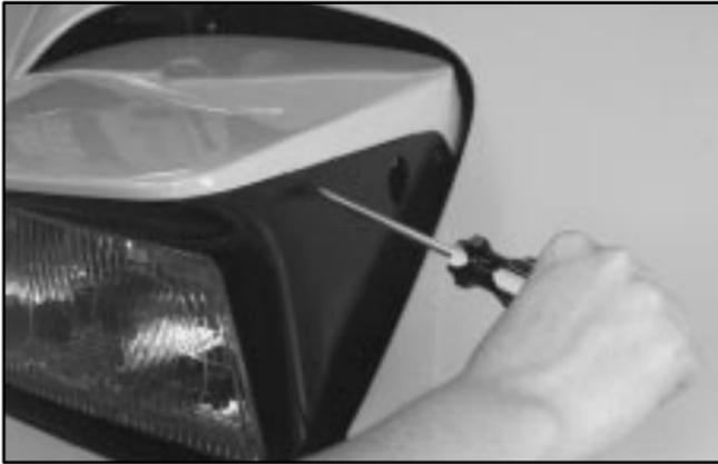
2. Remove the screws using a Phillips screwdriver on each side of the headlamp bezel.
