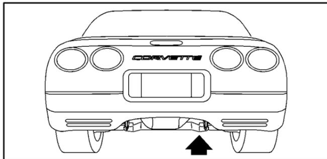
The rear lifting point can be accessed from the rear of the vehicle, on either the driver's or passenger's side.
