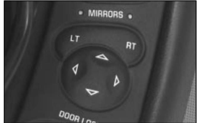
The electric mirror control is on the driver's door. It controls the driver's and passenger's mirrors. To adjust either mirror, press the LT (left) or RT (right) button to select the mirror, then press the arrows to adjust the direction of the mirror. The selected mirror will stay on for 20 seconds after the last adjustment. An indicator light will come on above the mirror that you select.
