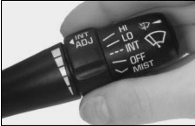
You can control the windshield wipers by moving the lever with the wiper symbol on it. This lever is located on the right-hand side of the steering column.
