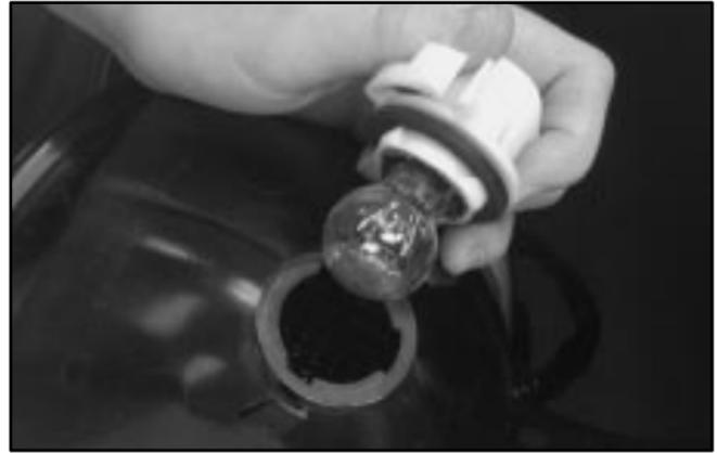
4. Remove the bulb from the socket.
