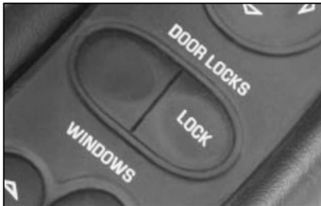
Press the power door unlock/lock switch on either door to unlock or lock both doors at once.
