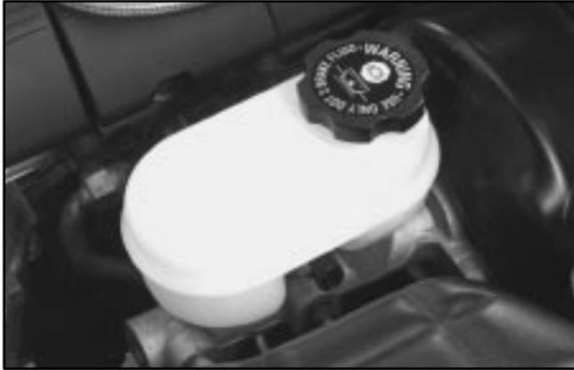
Your brake master cylinder reservoir is on the driver's side of the engine compartment. It is filled with DOT-3 brake fluid.
