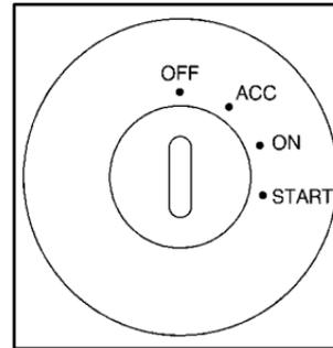
With the key in the ignition switch, you can turn the switch to four positions.
