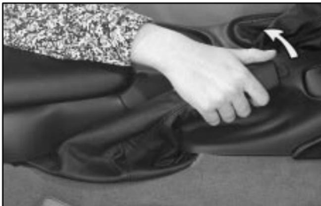
To set the parking brake, hold the brake pedal down. Pull the parking brake lever up. This sets your parking brake. If the ignition is on, the brake system warning light will come on.
