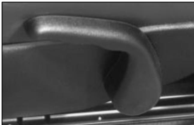
The lever for the reclining seatback is located on the side of each seat, near the base.
