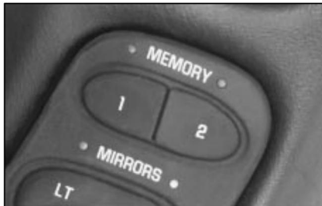
MEMORY can store and recall the settings for the driver's seat position, the outside rearview mirror positions, telescopic steering wheel (if equipped), radio presets, tone, volume, playback mode (AM/FM, tape or CD), last displayed station, compact disc position and tape direction and climate control settings.
