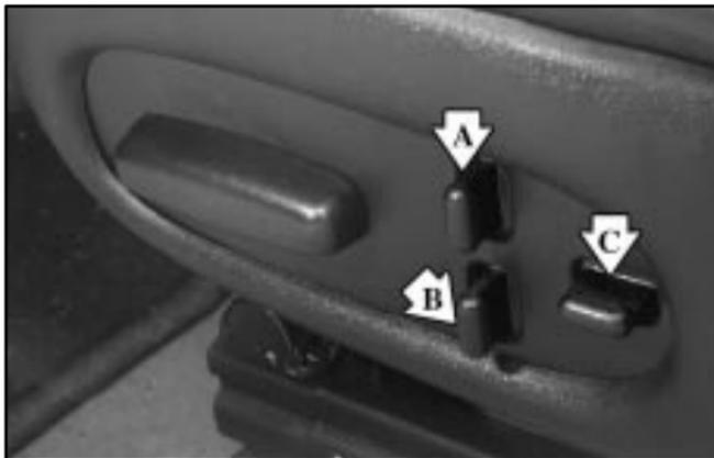
If your vehicle is equipped with a sport seat, there are three other switches that help you change the shape of the seat in addition to the power seat control. There are two lumbar supports for the middle (A) and lower (B) back. There's also a side bolster switch (C) that adjusts the sides of the seat around you to give you more lateral support.
