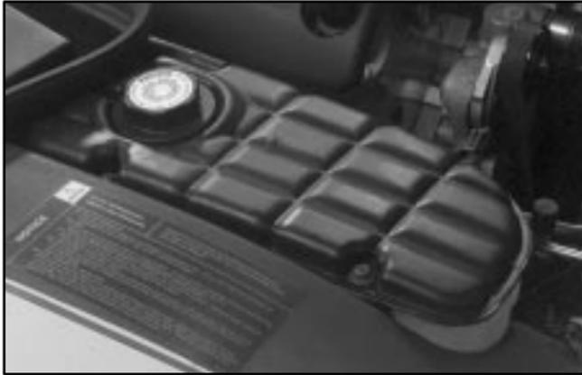
The coolant surge tank is located in the engine compartment behind the passenger's side headlamp.
