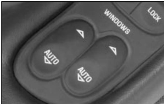
Both the driver's and passenger's window switches have the express-down feature. Tap AUTO and immediately release. The window will lower completely. To stop the express-down feature from lowering the window completely, simply tap the switch again.
