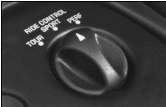
This switch is located on the center console. Turn it to select the suspension characteristic of your choice.
