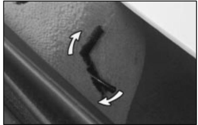
4. Gently lower the roof panel onto the carpeted ledge. Then, pull each release rearward and upward to place the storage pins into the holes of the roof panel.
