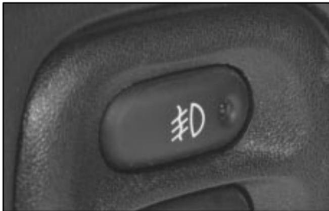
Use the fog lamps for better vision in foggy or misty conditions. Your parking lamps or low-beam headlamps must be on or the fog lamps won't work.
