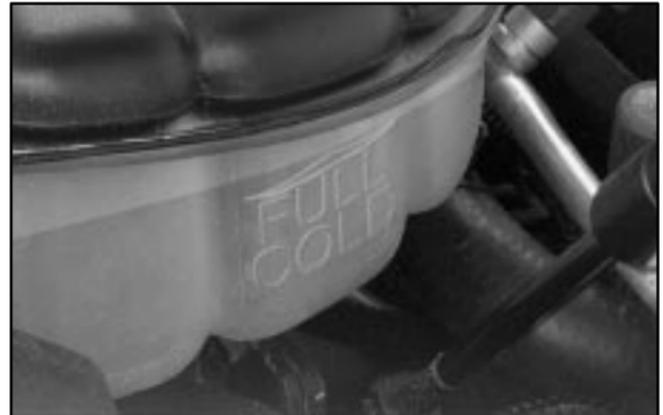
When the engine is cold, the coolant level should be at or above the FULL COLD mark. If it isn't, you may have a leak in the radiator hoses, heater hoses, radiator, water pump or somewhere else in the cooling system.
