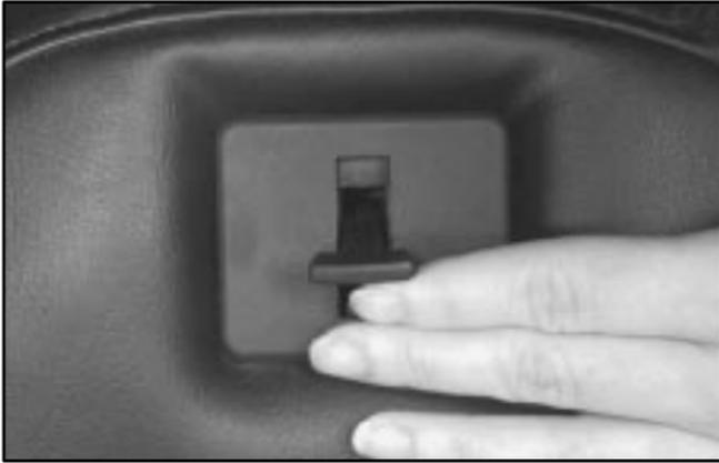
Both seatbacks fold forward to give you access to the rear area. To fold a seatback forward, lift this latch, which is located on top of the backside of the seat, and pull the seatback forward. The seatback will lock down in this position. To unlock, lift up on the latch and push the seatback rearward. When you return the seatback to its original position, make sure the seatback is locked.
