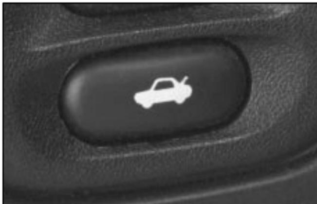
To use the hatch/trunk lid release on automatic transmission vehicles, your vehicle must be in PARK (P) or NEUTRAL (N). For manual transmissions, set the parking brake. See "Parking Brake" in the Index.
