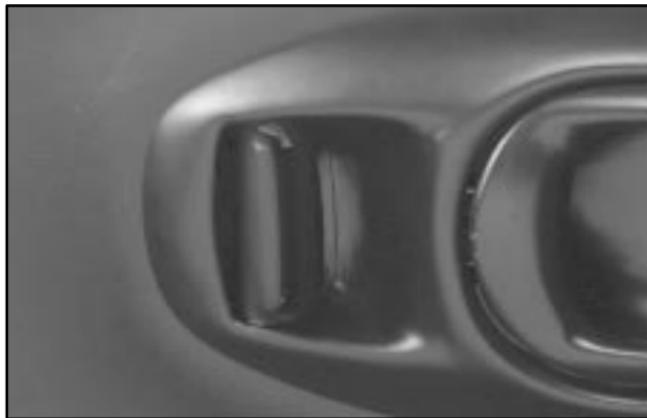
To lock the door from the inside, move the manual lock control located on the door forward. To unlock it, move the lock control on the door backward.
