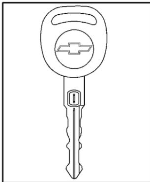
Your vehicle is equipped with the PASS-Key (Personalized Automotive Security System) theft-deterrent system. PASS-Key is a passive theft-deterrent system. It works when you insert or remove the key from the ignition.
