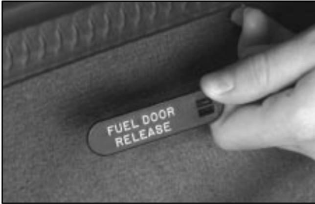
If your fuel filler door release won't operate, there is a manual release tab. The tab is located against the upper trim on the driver's side in the rear compartment.
