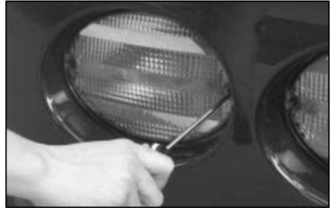
1. Remove the screws using a Torx<sup>®</sup> screwdriver.
