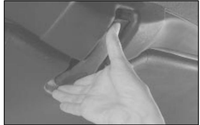
6. To unlock the rear of the roof panel, press the latch release button with your thumb and pull down the latch lever with your fingers.
