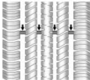
One way to tell when it is time for new tires is to check the treadwear indicators, which appear when the tires have only 1/16 inch (1.6 mm) or less of tread remaining.
