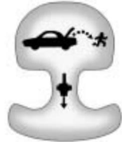
There is an emergency trunk release handle located inside the trunk on the trunk latch. On some vehicles, the release handle can be accessed by folding the rear seat center seatback. See *Rear Seats* on page 2-6. Pull the release handle to open the trunk from the inside.
