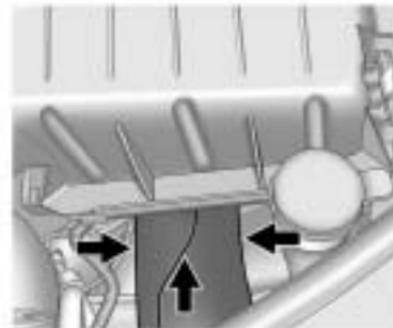
2. Press in on the tabs located on the sides of the duct and then push the duct rearward into the air cleaner/filter housing.
