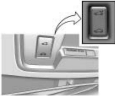
The sunroof can be opened without holding the switch down. Push the switch in the open direction until the second pause. The sunroof will fully open.
