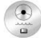
The power steering fluid reservoir is located under the engine cover on the driver side toward the front of the engine compartment. See *Engine Compartment Overview* on page 9-6.
