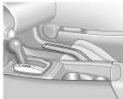
To apply the parking brake, pull up on the parking brake handle. It is not necessary to push in on the release button while applying the parking brake. If the ignition is in the ON/RUN position, the brake system warning light will come on. See *Brake System Warning Light* on page 4-22.
