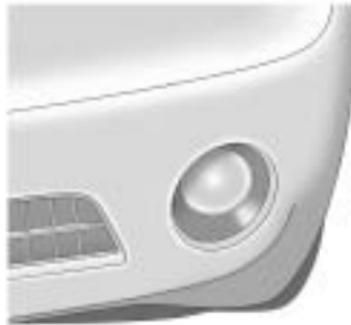
1. Locate the bulb assembly under the front facia.
