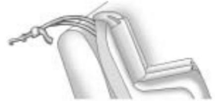
If the position you are using does not have a headrest or head restraint and you are using a dual tether, route the tether over the seatback.
