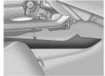
2. Pull the passenger side console trim away from the front half of the console to expose the shifter mechanism.
