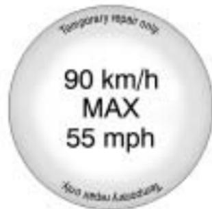
16. If the flat tire was able to inflate to the recommended inflation pressure, remove the maximum speed label from the sealant canister and place it in a highly visible location. The label is a reminder not to exceed 90 km/h (55 mph) until the damaged tire is repaired or replaced.
