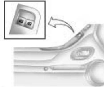
The power window switches located on the driver door control all windows. The window switches on the passenger door are only for that window. Push the front of the switch down to open the window. Pull the switch up to close it.
