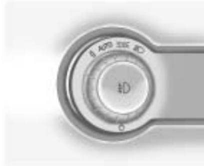
The exterior lamps control is located on the instrument panel, on the outboard side of the steering wheel.
