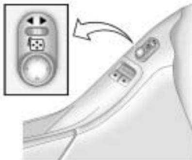
Vehicles with outside power mirrors have controls located on the driver door armrest.
