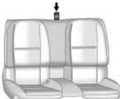
1. Pull on the strap located on the top of the of the rear seatback.
