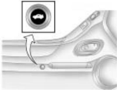
From inside the vehicle, press the
