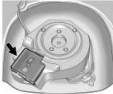
This vehicle may have a tire sealant and compressor kit in place of a jack or spare tire. It is located in a foam container in the trunk.
