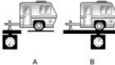
The trailer tongue (A) should weigh 10 to 15 percent of the total loaded trailer weight (B).
