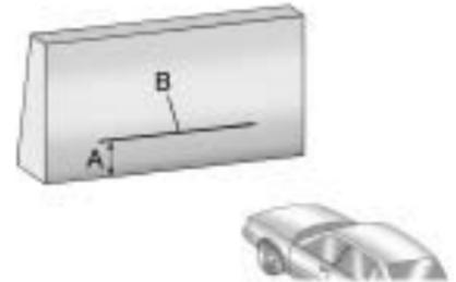
4. At the wall measure from the ground upward (A) to the recorded distance from Step 3 and mark it.
