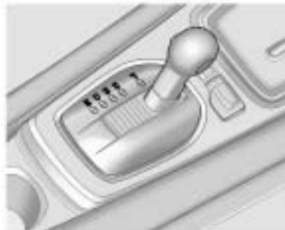
**P (Park):** This position locks the rear wheels. It is the best position to use when starting the engine because the vehicle cannot move easily.
