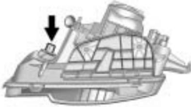
3. Disconnect the wiring harness and turn the bulb socket counterclockwise to remove it from the headlamp assembly.
