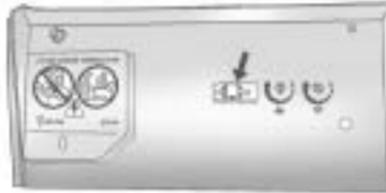
4. After Steps 1 through 3 have been completed, locate inside the garage the garage door opener receiver (motor-head unit). Locate the “Learn” or “Smart” button. The name and color of the button may vary by manufacturer.
