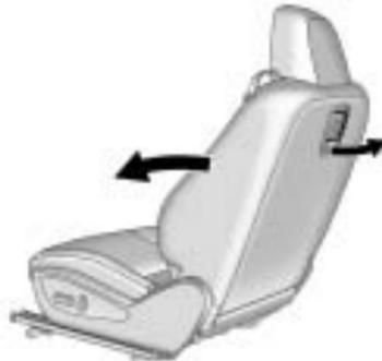
To access the rear seats pull up on the latch, located on the rear of the driver or front passenger seatback. Fold the seatback forward.
