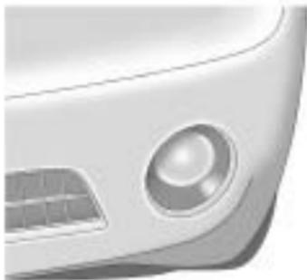
1. Locate the bulb assembly under the front fascia.
