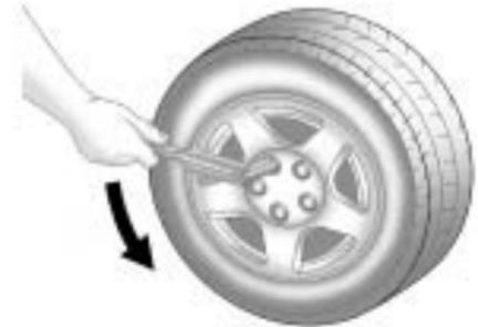
2. Use the fully extended wheel wrench to loosen all the wheel nuts one-half turn counterclockwise. Do not remove them.
