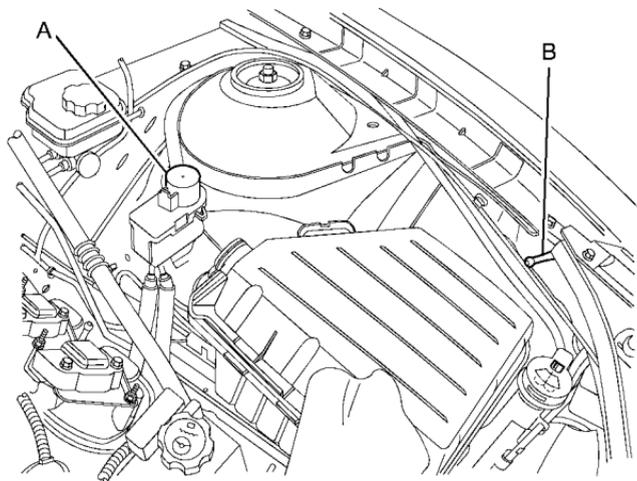
The jump start positive (A) and negative (B) posts are located in the engine compartment on the driver side of the vehicle.
