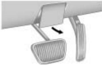
1. Pull the release handle that is located below the instrument panel to the left of the steering wheel.
