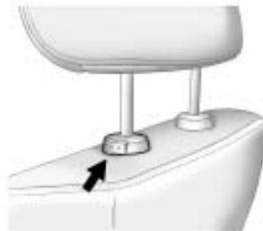
Pull the head restraint up to raise it. To lower the head restraint, press the button, located on the top of the seatback, and push the restraint down.
