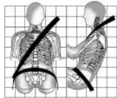
Sit up straight and always keep your feet on the floor in front of you. The lap part of the belt should be worn low and snug on the hips, just touching the thighs.
