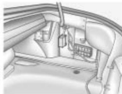
The rear compartment fuse block is located on the right side of the trunk behind a cover. Remove the six convenience net retainers, the rear sill plate, and the two passenger side trim retainers, then swing the trim out of the way.
