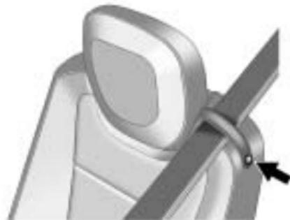
1. If the seat has a safety belt guide, and the safety belt is not routed through the guide, snap the guide around the belt webbing. Be sure the belt is not twisted.
