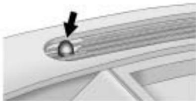
The security light is located on the instrument panel.
