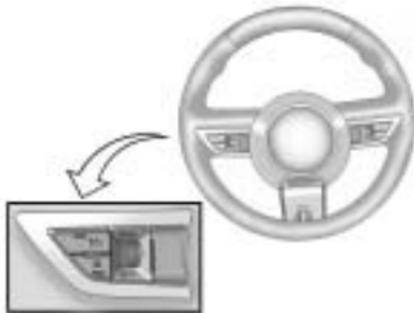
The cruise control buttons are located on the outboard side of the steering wheel.
