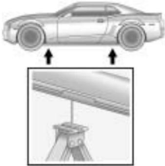
3. Position the jack lift head at the jack location nearest the flat tire. The location is indicated by a mark on the bottom edge of the vehicle. The jack must not be used in any other position.
