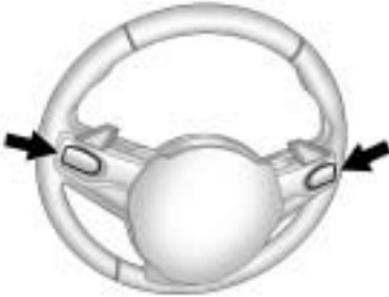
Tap Shift allows the driver to manually control the automatic transmission. To use Tap Shift, the shift lever must be in M (Manual Mode). Vehicles with this feature have flags on the top of the steering wheel to indicate to the driver the location of the switches on the back of the steering wheel. Tap the left
