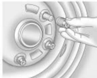
8. Remove all of the wheel nuts and place them in a dry, clean place to avoid getting dirt in the threads.
