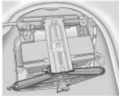
1. The jack and tools are stored below the spare tire. Remove the jack from the retaining bracket.
