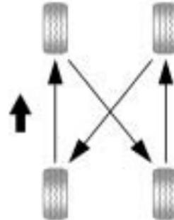
When rotating the vehicle's tires, always use the correct rotation pattern shown here.
