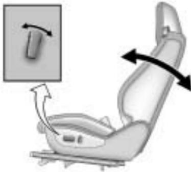
On vehicles with power reclining seatbacks the control is located on the outboard side of the seat.
