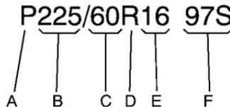
**(A) Passenger (P-Metric) Tire:** The United States version of a metric tire sizing system. The letter P as the first character in the tire size means a passenger vehicle tire engineered to standards set by the U.S. Tire and Rim Association.
