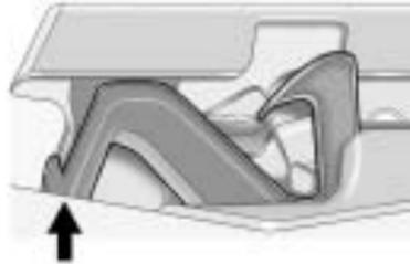
2. Pull up on the secondary hood release. The lever is located near the middle of the hood.
