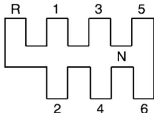
These are the shift patterns for the six-speed manual transmissions.
