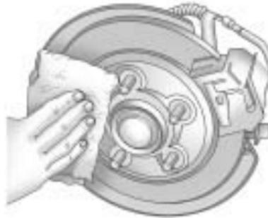
9. Remove any rust or dirt from the wheel bolts, mounting surfaces and spare wheel.
