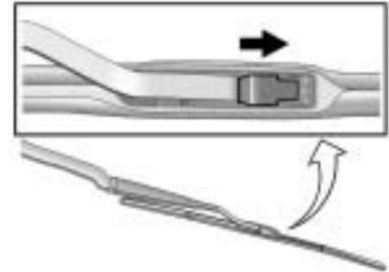
2. Lift up on the latch in the middle of the wiper blade where the wiper arm attaches.
