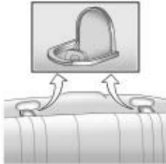
The top tether anchors are located on the rear seatback filler panel. Be sure to use an anchor located on the same side of the vehicle as the seating position where the child restraint will be placed.
