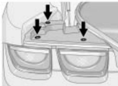
2. Remove the close out panel retainers to gain access to the bulb socket connectors.
