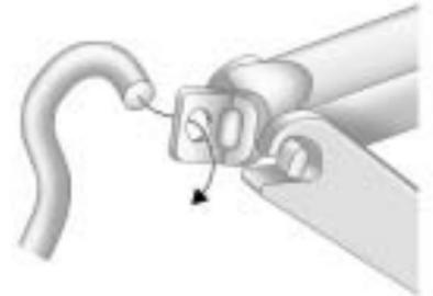
5. Fit the jack handle extension onto the jack by sliding the hook through the end of the jack.
