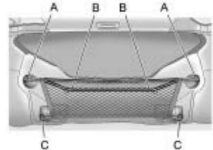
The upper (A) and lower (C) hooks on each side of the trunk opening are provided to attach the net.
