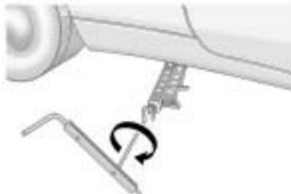
7. Raise the vehicle by turning the jack handle extension clockwise until the vehicle is far enough off the ground to allow enough room for the compact spare tire to fit under the vehicle. Keep the hook parallel to the ground. The wrench may need to be removed and repositioned to continue turning it.
