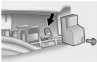
3. Remove the retainer and the shift lock manual release cover.
